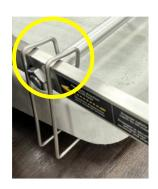
**SECOND STEP,** install all 4 pad hangers as shown. It helps to lift up slightly on the steel base.
