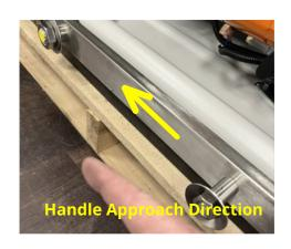
step 3: Line up handle with base. The handle must always approach the base fulcrum (bolt with yellow label) from the latch end of the base. Once the fulcrum is fully engaged onto both of the handle's front hooks, press down on the handle with enough force to lock both of the rear latches. Then you may move the load. If you need to approach the generator from the other end, just swap the side rails to the other sides.
