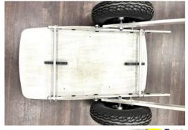
**THIRD STEP,** slide the locking wedges under the center of each bar hard enough to lock in the position of the base over the pad. NOTE the orientation of the locking wedges in this picture are for a 4" Generac pad. For the 3" pads, flip the locking wedges over.
