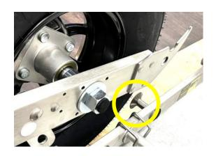
FORTH STEP, approach the pad with the cart handle level to the ground. This is so the handle's front fulcrum hooks can get over the pad lifting hooks. Once the handle's front fulcrum hooks are a few inches from the base fulcrum bolts, lift the handle and slide the handle's hooks to fully engage the fulcrum bolts. Then press down on the handle to lock in the handle's rear latches.
