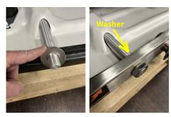
STEP 2: Attach rails to lifting rods. First slide on one washer on each end of the rods, then align the base rail holes with the round base rods, and loosely attach a nut on each rod end. Finish by hand tightening all 4 nuts. See hole chart for generator being moved.
