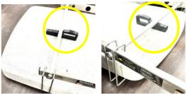
DO NOT ATTEMPT TO LIFT THE PAD WITHOUT BOTH OF THE WEDGES FIRMLY IN PLACE.
